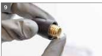
9 Grease thread of material flow control screw
