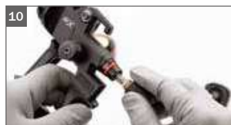
10 Installing material flow regulation screw
