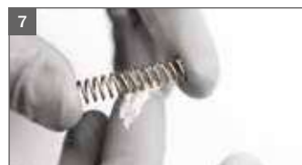
7 Grease and insert paint needle spring
