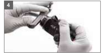
4 Alternatively, the integrated tool within the trigger can be used.
