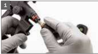
1 First remove paint needle.
