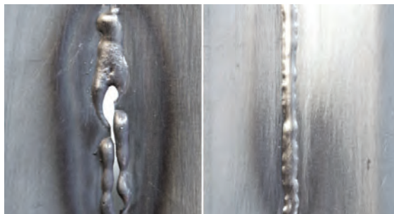
Ideal for sectional repairs with MIG-weld-seams
