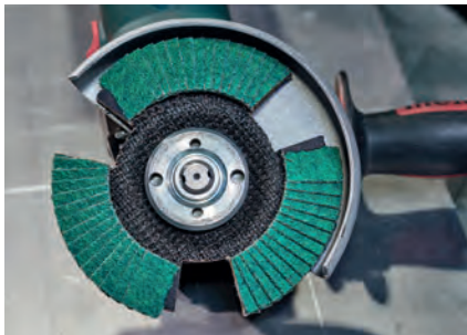
Three clever cut-outs for an unobstructed view of the workpiece...
