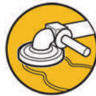
Spread compound and polish at 1,200–2,000 rpm
