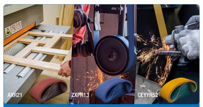
3 new versions of Endless Belts for various grinding applications. AXR21 with X Poly-Cotton backing and Aluminum Oxide abrasive grain for wide belts in wood industry, ZXPR13 with X Heavy Poly-Cotton backing and Zirconia for narrow belts in various metal industries and CEYYR52 with Y Polyester backing and Ceramic-Zirconia abrasive grain for narrow belts in heavy metal grinding applications.
